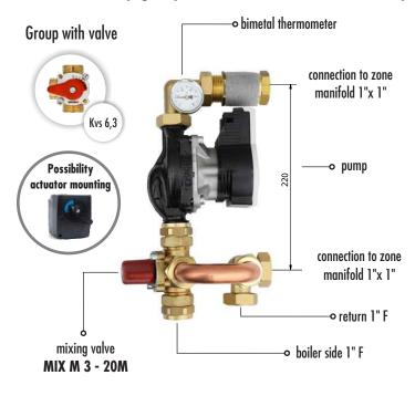
Mixing group **M-SMT - DN 20** with a rotary valve is designed for floor heating manifolds. Its task is to limit the temperature of the medium introduced into the manifold. The group can be connected using a nipple (see table below) with all types of brass manifolds. The set consists of a rotary mixing valve with a flow of kvs 6.3 with the possibility of connecting the actuator **MP 10**, thermometer for supply water, brass connection couplings and Wilo or Grundfos pumps.
